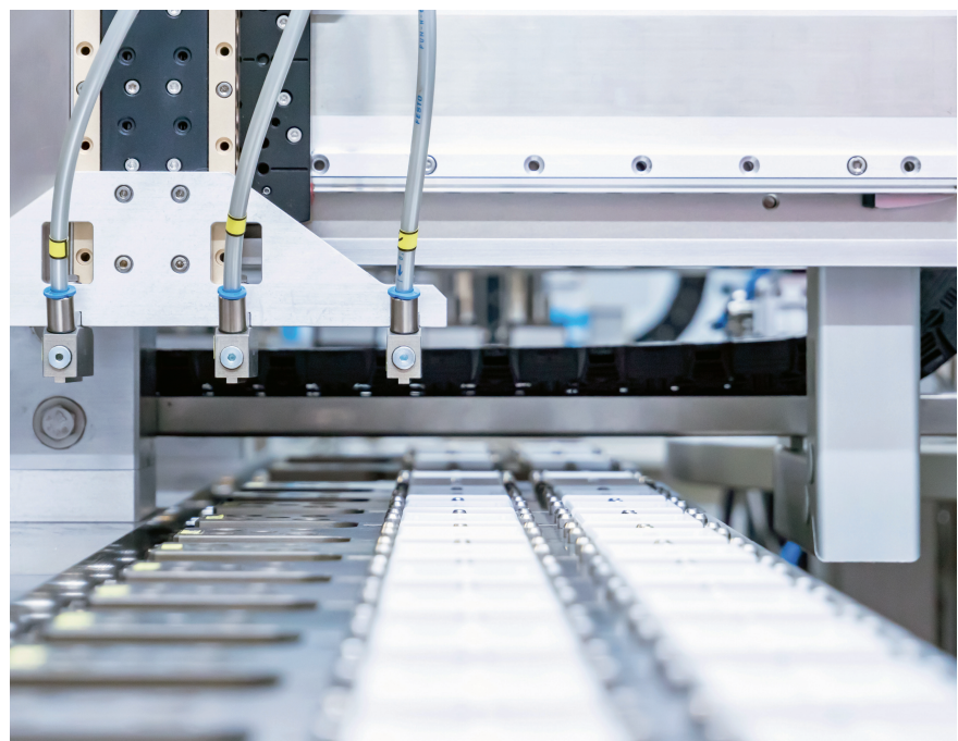
Assembly time 750 ms: the rapid transport of individual parts – here the lower shells – is the prerequisite. © MA micro automation
