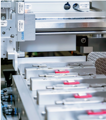
Cutting station: it makes individual test strips from card material and automatically sorts out faulty parts. © MA micro automation
